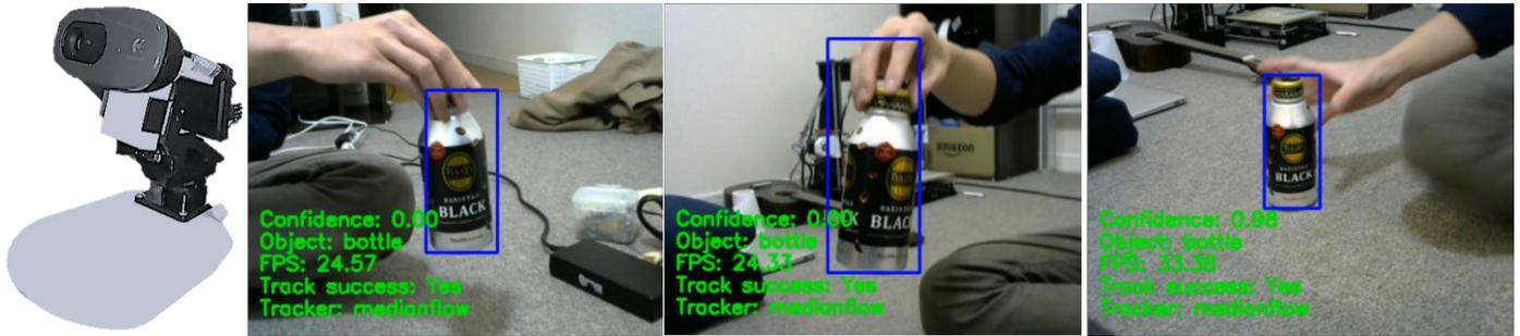
Figure 48: Pan-tilt module with tracker test
