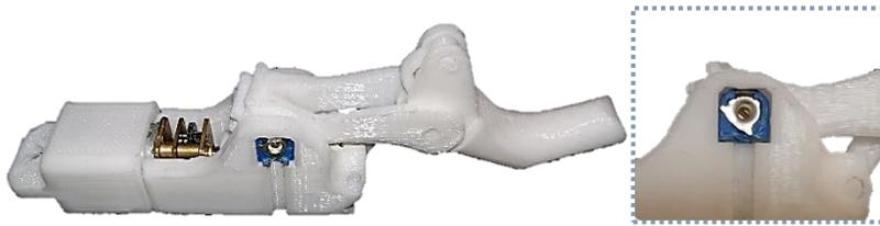
Figure 10: Finger module printed with encoder
