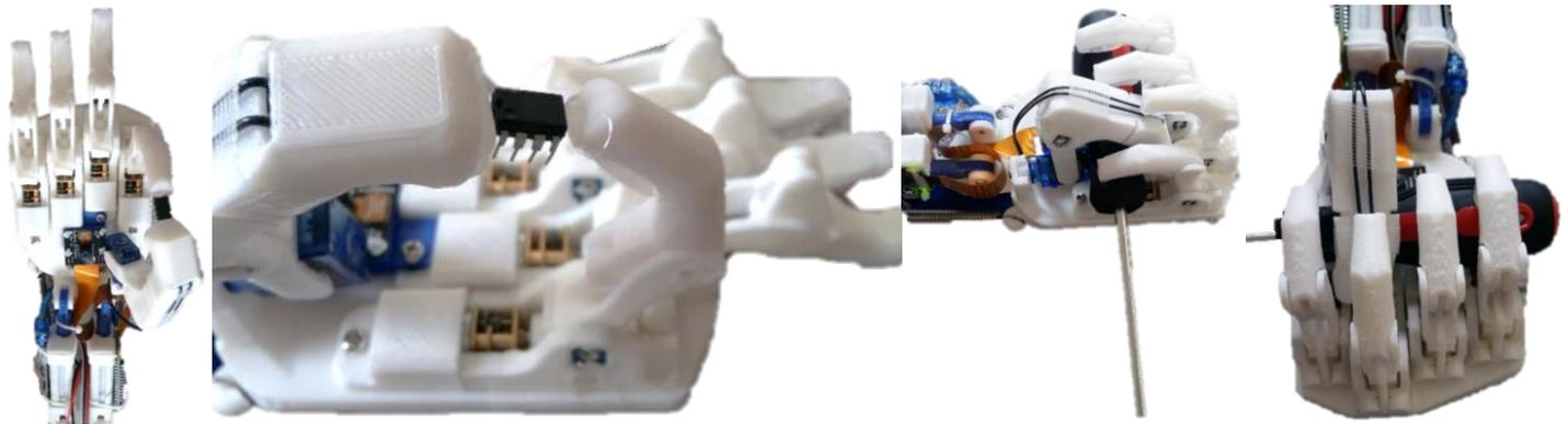
Figure 27: Tip pinch grip (microchip) and random grip (screwdriver)
