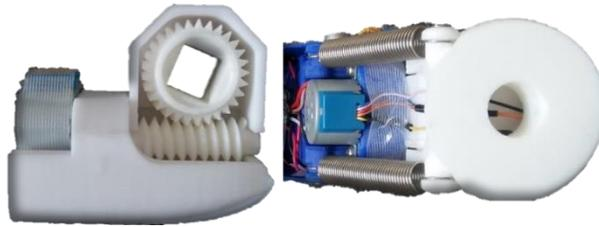
Figure 23: Elbow gear box and springs
