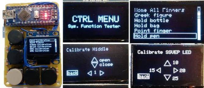
Figure 28: First version of watchdog timer with button and OLED interface
