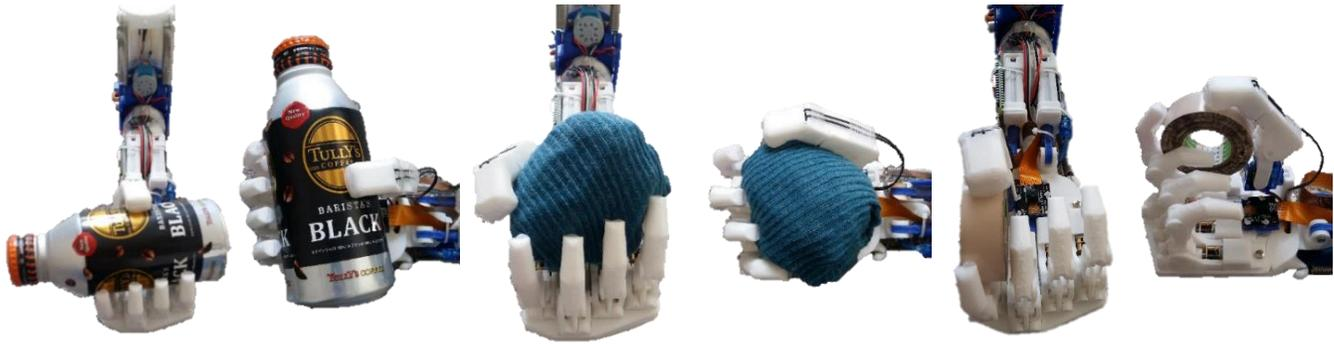
Figure 25: Cylindrical grip (bottle), spherical grip (ball) and tripod grip (tape roll)
