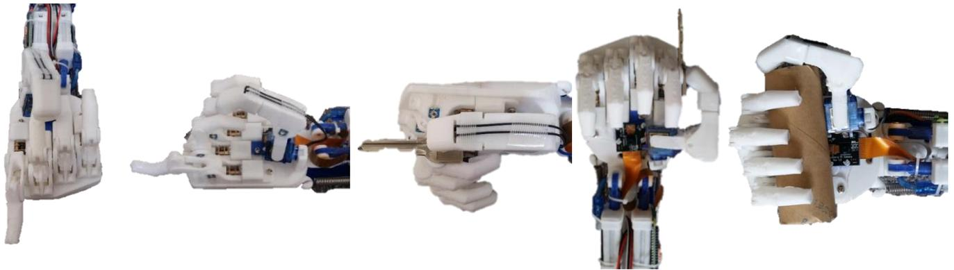
Figure 26: Point grip, lateral grip (key) and hook grip (paper roll)
